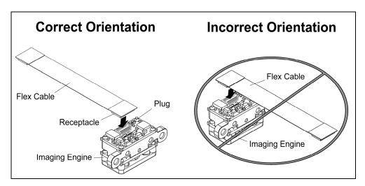
Figure 39. Flex Cable Orientation – Imaging Engine
